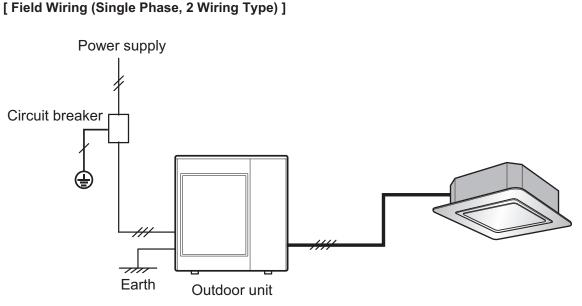
This figure is representative example for field wiring. Actual appearance of outdoor and indoor units could be different with installed product.
