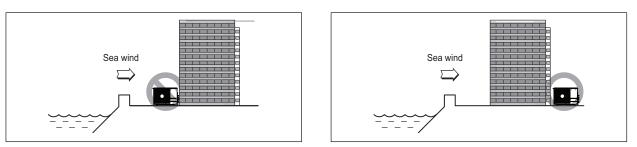
2. In case, to install the outdoor unit on the seaside, set up a windbreak not to be exposed to the sea wind.
