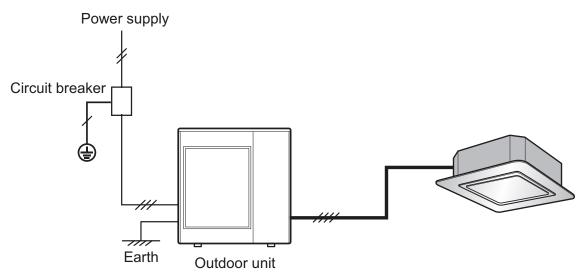
X This figure is representative example for field wiring. Actual appearance of outdoor and indoor units could be different with installed product.
