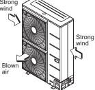
Turn the air outlet side toward the building's wall, fence or windbreak screen.
