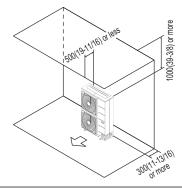
• Obstacle on the air intake side, and both sides
