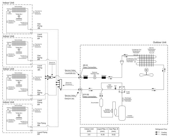
1. The pipes between the indoor units and the branch kits must have same dimensions as indoor unit connections
