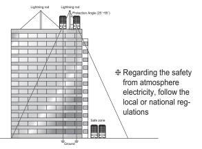
1. To protect outdoor unit from lightning, it should be placed within lightning safety zone.
